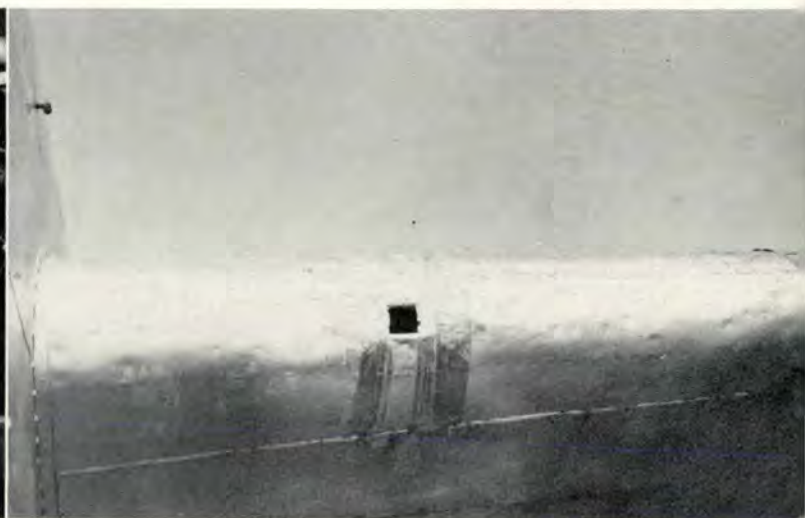
Speed is an important factor, but size of the hailstone has the greatest effect in damage, such as to F-51 above and B-25 below
