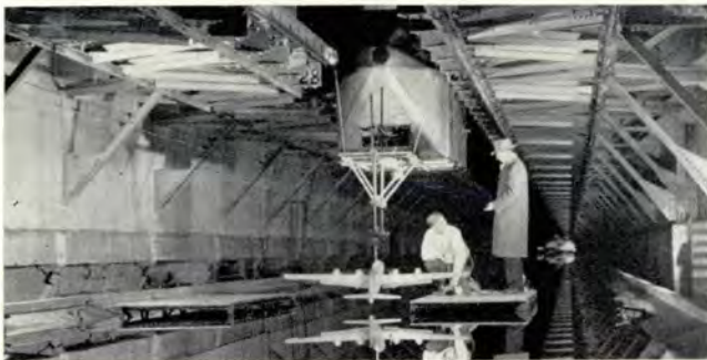
A B-29 ditching model being set up for a test in tank at Langley. Blewo, a scale model is filmed and studied for spin characteristics
